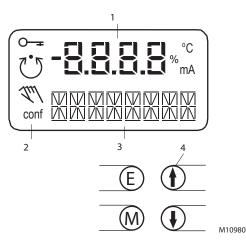
Fig. 1: LCD display with operating buttons
